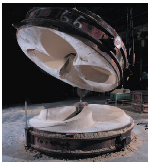
The use of “no bake” sand in molding larger Michigan Propeller patterns results in accurate castings.
