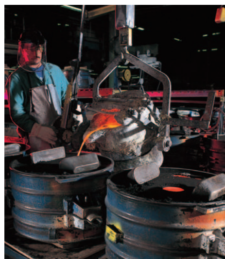
Melt temperatures are critical, and tightly controlled on the special alloys used in Michigan Propellers foundry.
