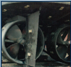
Typical nozzle installations
