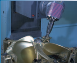
Computer driven CNC machine mill certain FEDERAL custom propellers exactly and consistently.
