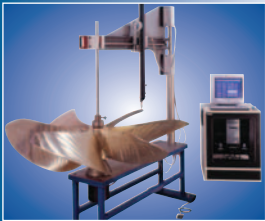
Sophisticated measurement recording instruments (Halé MRI) facilitate full documentation and perpetual record.
