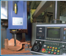
All patterns are machined cut on computer driven CNC cutting mills. This assures that the design criteria will carry through to the propeller castings.
