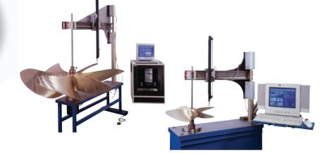
In process and final inspection with gauges, pitchometer, and computerized inspection (MRI), equipment insures production accuracy. Computer generated carton labels, keyed off the part number, accurately identify critical information on each propeller that is packed.
