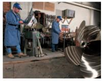
Each hand-crafted or machine finished propeller blade is templated, and each propeller is checked for pitch, spacing and track in process, to insure accuracy of the final product. Balancing equipment is located and used in each step of the finishing process.
