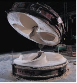
The use of "no bake" sand in molding larger Michigan Propeller patterns results in accurate castings.
